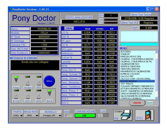
In particular verify communication status, error or warning messages and the correct operation of the MEASURE command.
